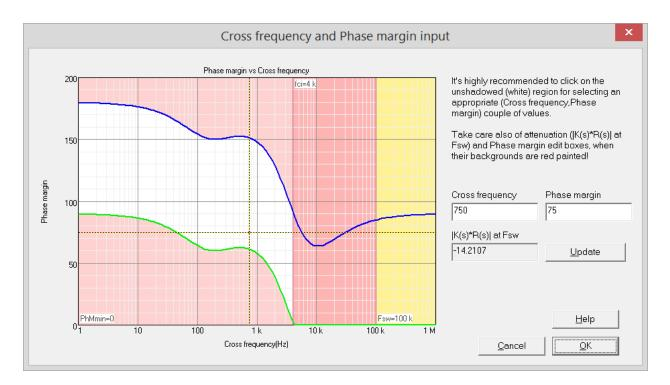
Now click OK to confirm the design, and the program will automatically show the performance of the system in terms of the frequency response, polar plot, transient response, etc.
