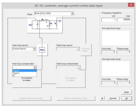
The type of regulator depends on the plant controlled. In this example, the proper choice is a Type 2 regulator. Select the Type 2 regulator, and enter the parameters as shown below.
