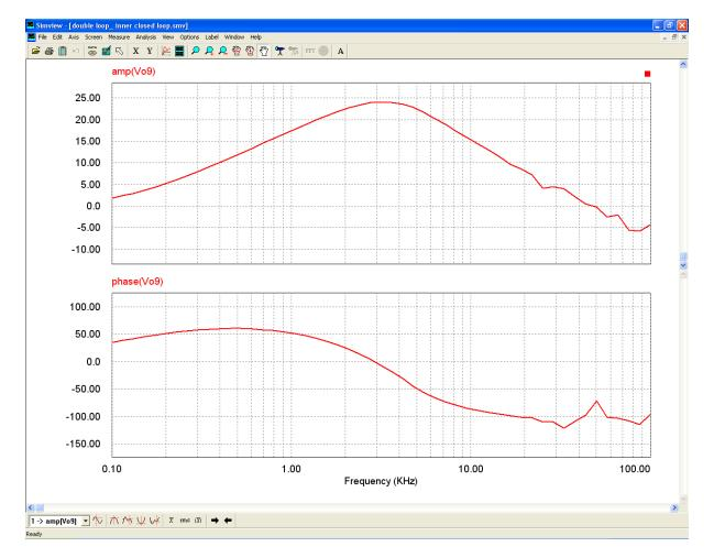
The frequency response can be easily compared to that obtained in SmartCtrl through the merge function in SmartCtrl. To do that, the PSIM ac sweep result must be saved as "tab separated text file (Excel compatible)". In this example, the PSIM ac sweep results are saved to a file called "inner closed loop.txt".
