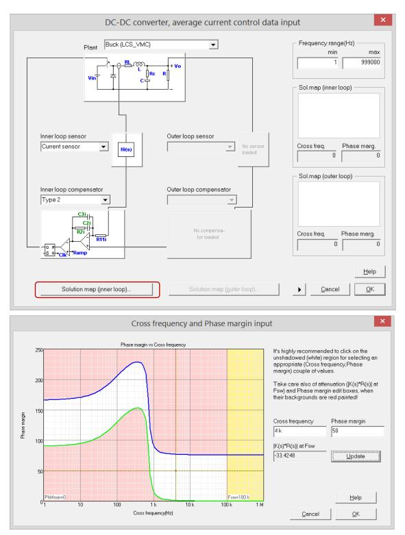
The x-axis of the Solution Map is the crossover frequency and the y-axis is the phase margin. Based on the converter parameters and the type of regulator selected, SmartCtrl will generate a safe esign area as shown in the white area in the Solution Map. Any selection of the crossover frequency and the phase margin that is within this white area will lead to a stable solution.
