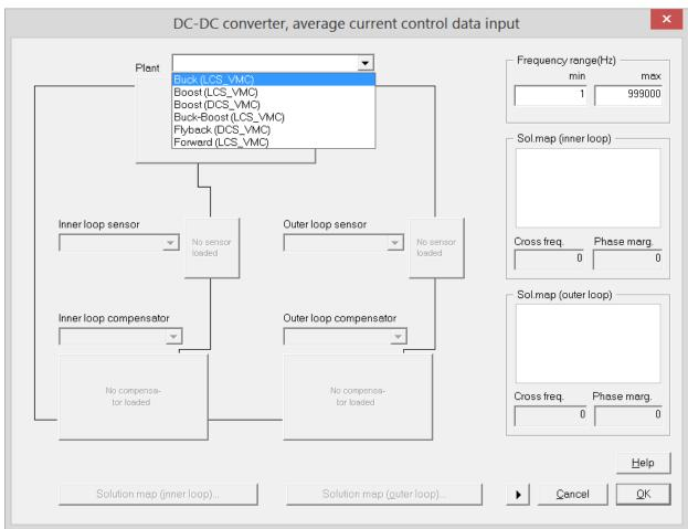
Similar to the single loop design, the double loop design must be done sequentially, and SmartCtrl will guide you through the process.
