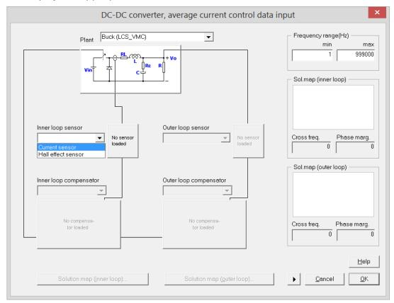
In this example, select **Current Sensor**, and specify the sensor gain, as shown below. Click OK to continue.
