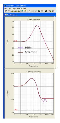
The green line corresponds to the results from PSIM ac analysis, and the red one is obtained by SmartCtrl. It can be seen that these two results compare well, especially in the low-frequency region.
