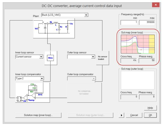
Click OK to complete the design of the inner current loop. One can move on to the outer voltage loop design.
